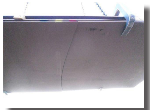
Example of a three point lift with a crack as an result.
